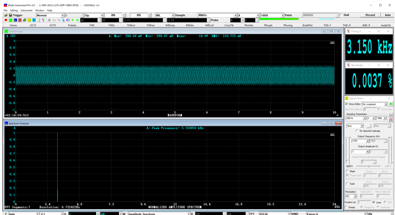
Fig. 10 Unweighted residual peak wow and flutter of a M-Audio Mobile Pre sound card measured through a loopback test
