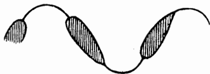
FIG. 5/2.—Oscillogram of shock-excited parasitic oscillation of extremely high frequency, carried on 50 cycle mains hum.
