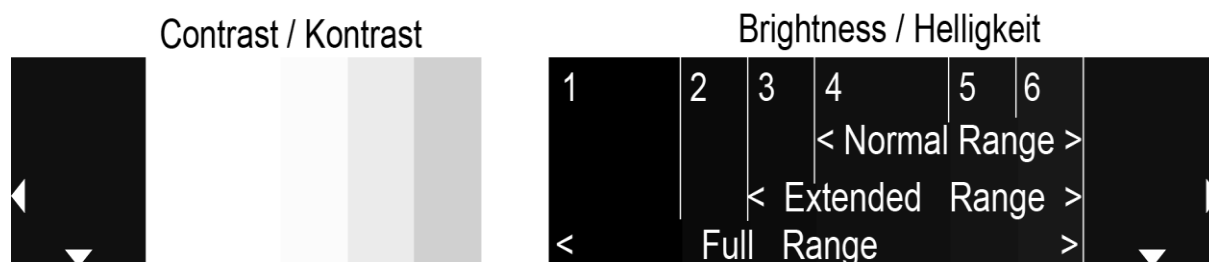
Figure 6.1.2.1 – The black levels - for adjusting the display brightness - can also be used to evaluate the video range of the signal.
