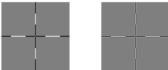
Figure 6.6.1 – Left – correctly set. Right - wrong settings (double contours visible)
