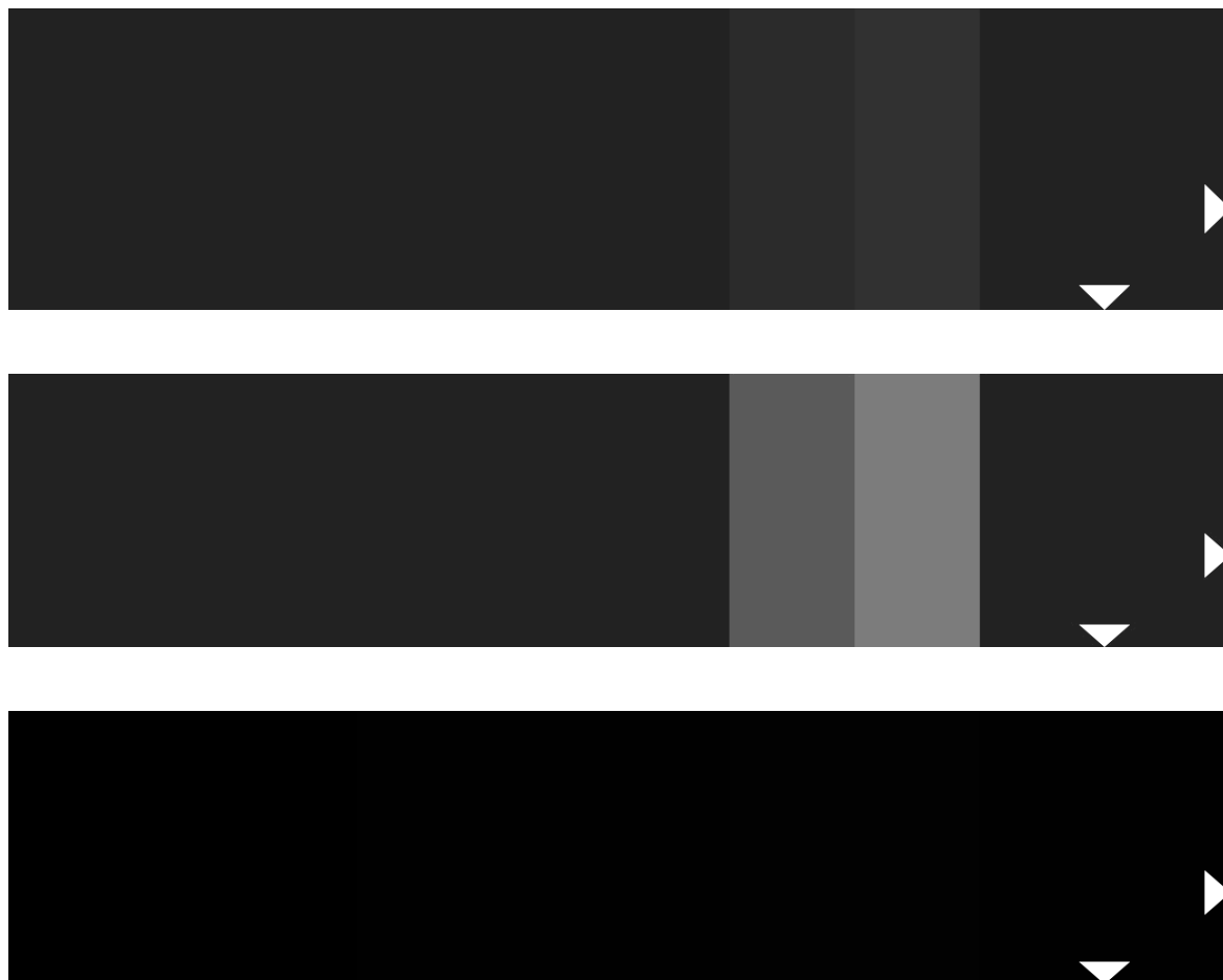
Figure 6.2.1.2 – Above: Here the brightness for normal range is adjusted properly. The bar 4 is minimally darker than the bar 5 and bar 6 is slightly brighter than the other bars. Middle: The bar 4, 5 and 6 differ significantly, and black (bar 3) appear gray. The brightness is set too high. Below: The bars 4, 5 and 6 are not discernible. The brightness is set too low.
