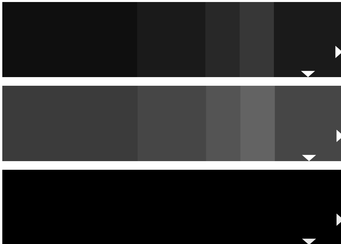
Figure 6.2.2.2 – Above: Here the brightness for extended range is adjusted properly. The bar 3 is minimally darker than the bar 4 and the bars 5 and 6 are slightly brighter than the other bars. Middle: The bars differ significantly, and black appears gray. The brightness is set too high. Below: The bars are not different in brightness. The brightness is set too low.
