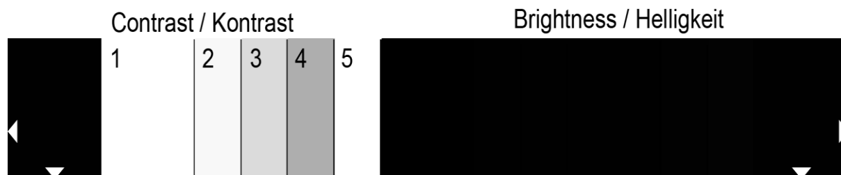
Figure 6.3.1 – The lower image area of the test pattern to adjust the contrast. The bars 1 to 5 are emphasized for the figure (white lines). Depending on the video range of your display you will see a similar or different representation.
