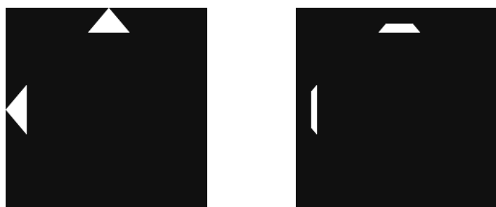
Figure 6.5.1 Ausschnitt – Left – correctly set. Right - wrong settings (overscan enabled)
