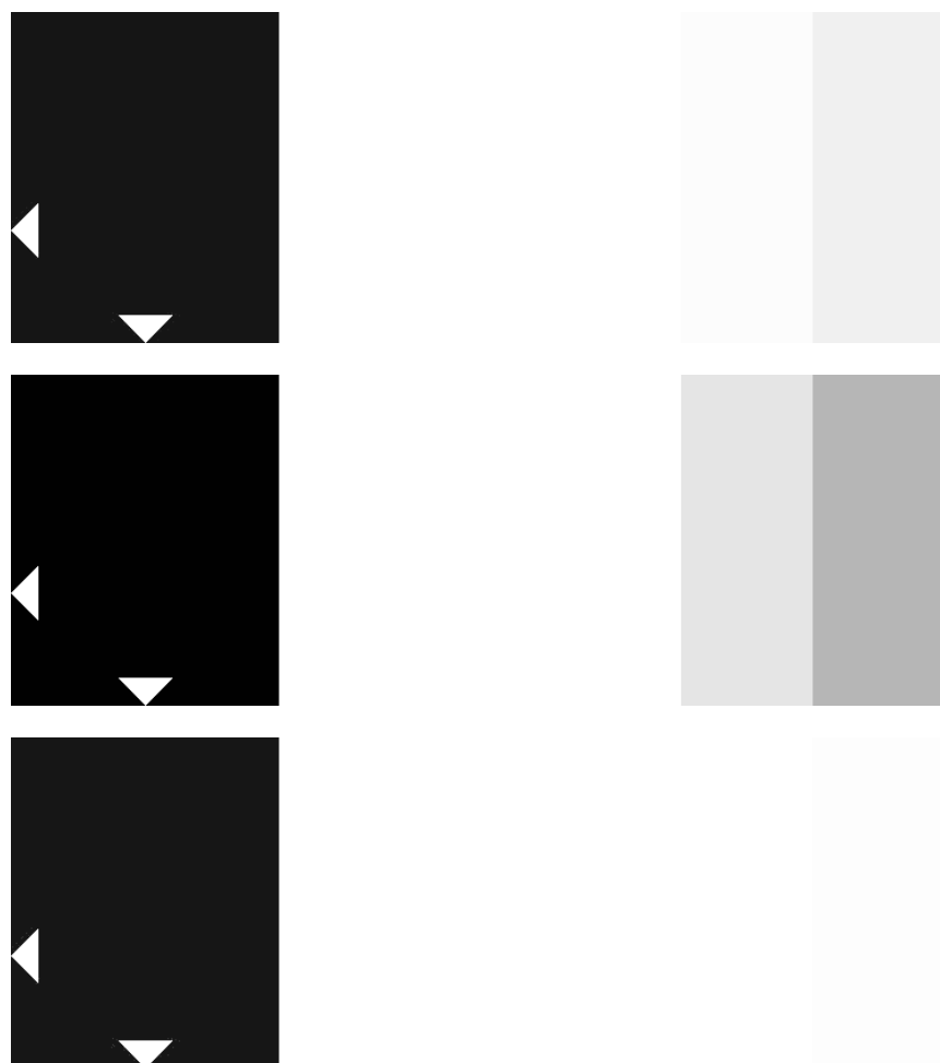
Figure 6.3.2.1 – Above: Here the contrast for extended range is adjusted properly. The bar 2 is minimally brighter than the bar 3. The bar 4 is slightly darker than the Bar 3. Middle: The bars vary significantly. The contrast value is set too low. Below: All the bars have the same brightness. You can't see any differences. The contrast value is set too high.
