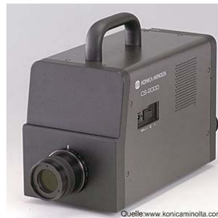
Spectroradiometer CS-2000 from KonicaMinolta
